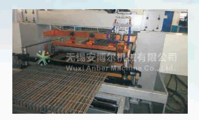
The machine adopts hydraulic device to control welding electrode; bar range: 2.5-5mm
