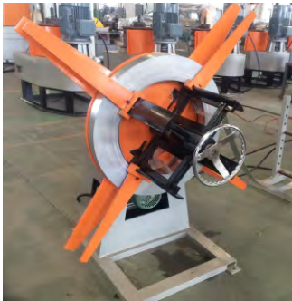
整条护角生产线包含5个部分：开料架，冲床，控制柜，成型，收料台 Seen on the picture, the “V” type angle bead production line consists of five parts: uncoiler, angle bead machine, electric control cabinet, roller profiling machine and collecting table.
