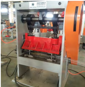
整条护角生产线包含5个部分：开料架，冲床，控制柜，成型，收料台 Seen on the picture, the “V” type angle bead production line consists of five parts: uncoiler, angle bead machine, electric control cabinet, roller profiling machine and collecting table.
