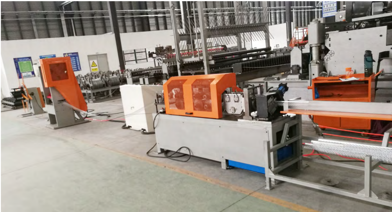
整条护角生产线包含5个部分：开料架，冲床，控制柜，成型，收料台 Seen on the picture, the “V” type angle bead production line consists of five parts: uncoiler, angle bead machine, electric control cabinet, roller profiling machine and collecting table.
